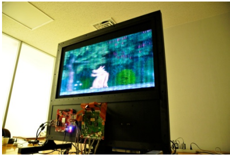
Figure 1. The 38-inch adaptive parallax autostereoscopic LED display
